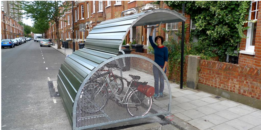
Figure 16 In-street cycle parking placed in the carriageway is one way to provide secure cycle parking at home. Attention should be paid to provide 30% of spaces suitable for adapted and inclusive cycle types such as trikes, cargo bikes and bike trailers © Cyclehoop
